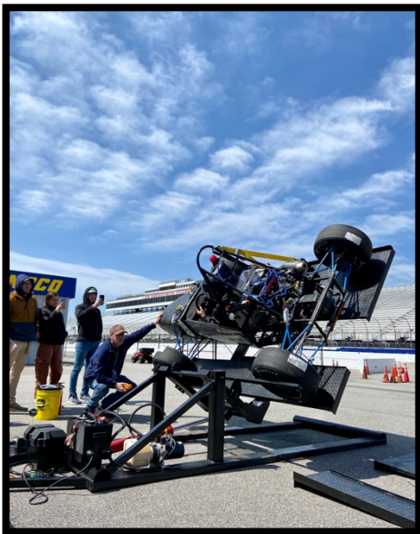
Middleberry's vehicle faces the formidable tilt test, a static event that tests rollover stability.
