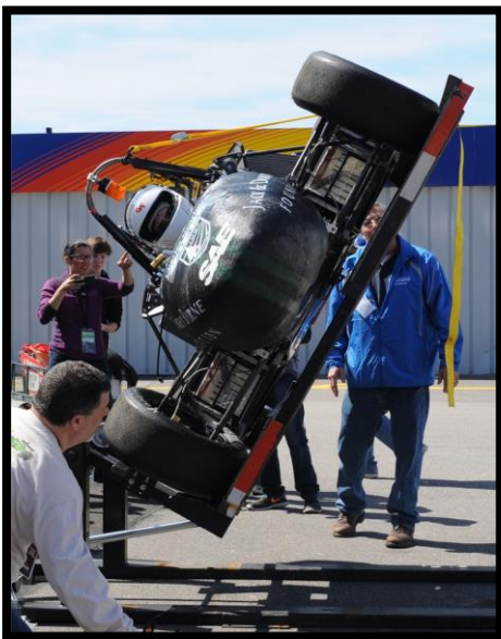
Dartmouth's vehicle faces the formidable tilt test, a static event that tests rollover stability.
